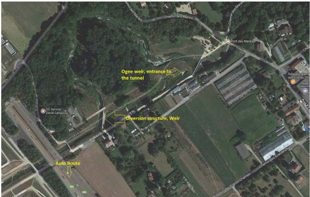
Figure 3 Newly constructed diversion structure and tunnel.
